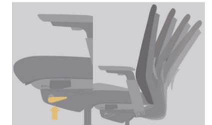
The pitch angle is adjusted to 4 gears. Adjustment range 22 degrees
